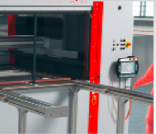
The manual lifting door or the high-speed door, which can be ordered as an option, safely separate the travel range of the linear robot from the operator.
