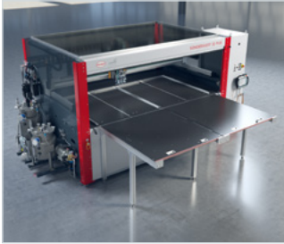
Shuttle table (optional): Two pick-up plates to be shifted manually in pendulum mode in one plane (can be connected to one pick-up plate for large parts)
