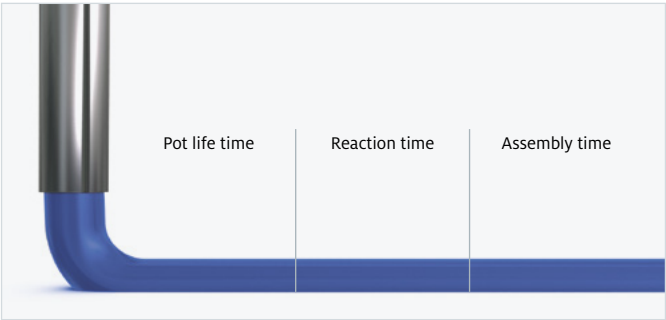
The different reaction phases of the polyurethane gel in chronological order
