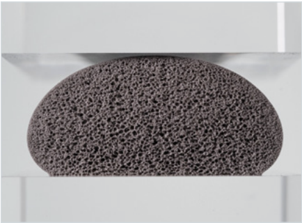
Cross-section of a polyurethane foam bead – uncompressed
