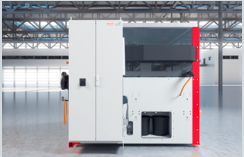
The front side (right) of the SONDERHOFF 3E FLEX dosing cell shows the switch cabinet attached to the cell chassis for controlling the dosing machine, to the left of which you see the holder for the MP 2 mobile panel, and to the right the opening for removing the filling shot and rinse water containers
