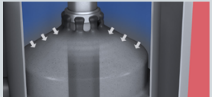
Material is continuously conveyed from the bottom of the pressure tank through a riser pipe and fed back onto the conical surface as a thin film. Due to the air loading, the density changes and the material becomes lighter in color.
