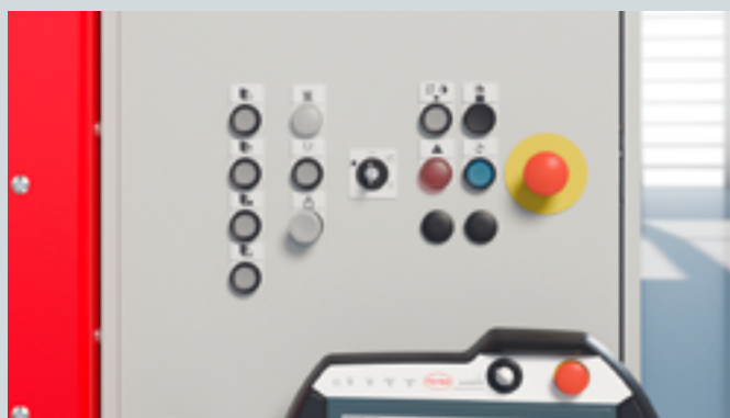
Operating mode control panel with warning lights, key switch for preselection of the operating mode, operating keys for high-speed door, and EMERGENCY STOP with proven Sonderhoff SAFETY concept.
