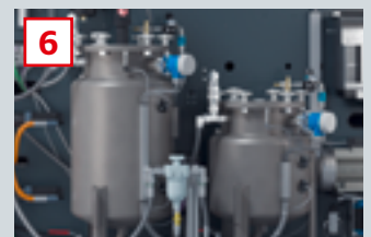
Material pressure tanks with optimized dimensions for asymmetrical (PUR systems) or symmetrical (SIL systems) mixing ratios
