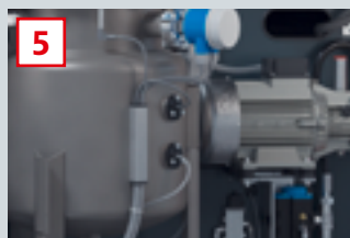
Capacitive sensors for filling level regulation
