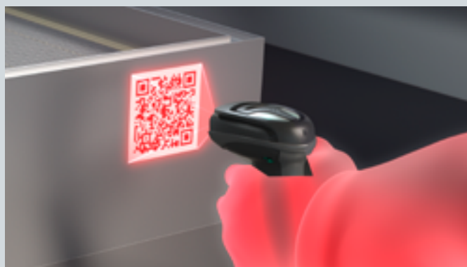
Hand-held scanner for selecting the CNC and dispensing program
