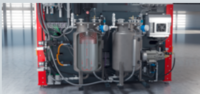
Material is continuously conveyed from the bottom of the pressure tank through a riser pipe and fed back onto the conical surface as a thin film. This process continuously reduces and completely dissolves air bubbles in the material.
