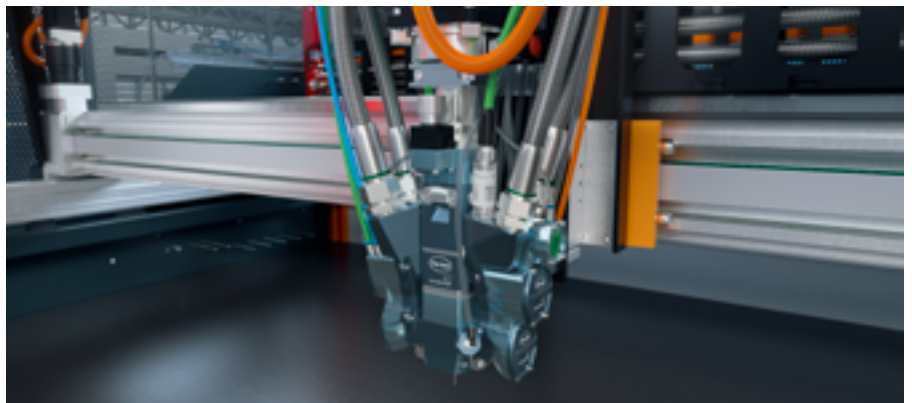
Standard equipment: Precision mixing head MK 800/825 PLUS for 2 components, with high-pressure water rinsing.
