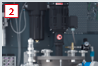
Agitator for homogenization of the A component
