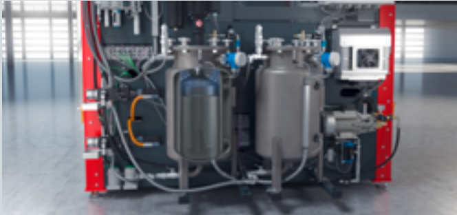
Compressed air cushion acts on material surface
