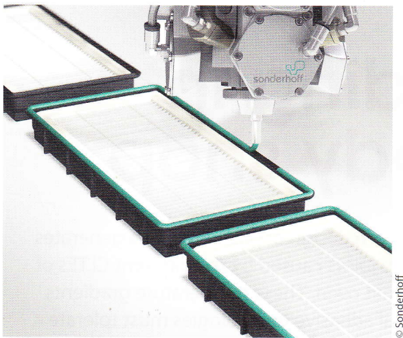
In order to ensure high-quality filter production, the adhesive and sealant must be precisely applied.
