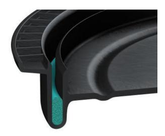
Fully automated, precise insertion of the FDA-compliant FERMAPOR® K31 PU foam seal into the groove of plastic drum lids with a Sonderhoff mixing and dosing system
