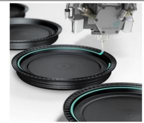
Fully automated, precise insertion of the FDA-compliant FERMAPOR K31 PU foam seal into the groove of plastic drum lids with a Sonderhoff mixing and dosing system.
