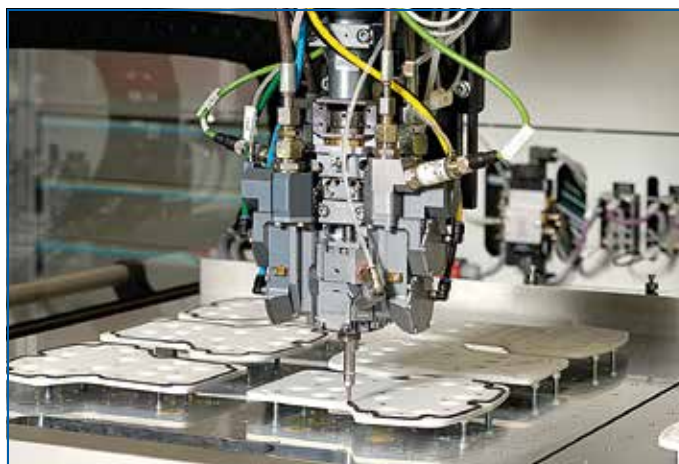
Two-component formed in-place foam gasketing with Fermapor K31 PU foam sealing
