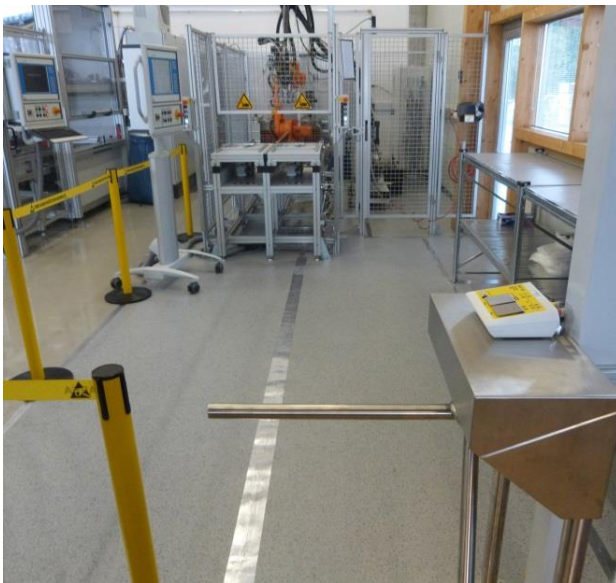
Certified ESD protection zone at the production of Sonderhoff PSA in Dornbirn, Austria
