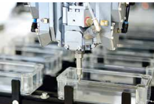
MK650 mixing head technology enables very narrow liquid foam gaskets to be applied directly on the part with all the advantages of the FIPFG process (© Sonderhoff)
