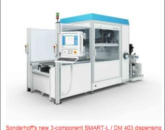
Sonderhoff's new 3-component SMART-L / DM 403 dispensin cell for foam sealing, gluing and potting of industrial parts
