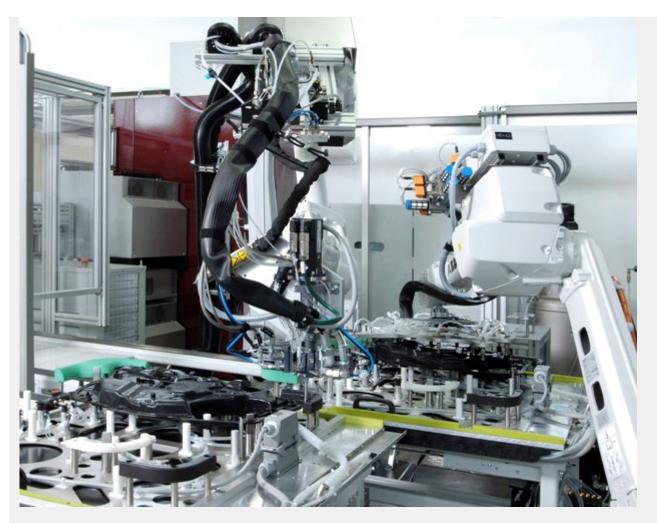
The mixing head attached to the articulated-arm robot precisely travels along the component contour for the sealing application (source: Sonderhoff Group)
