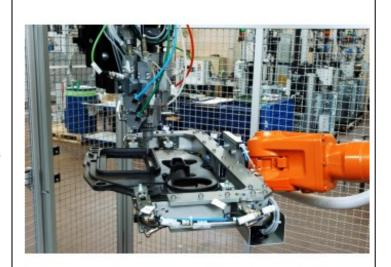
During Sonderhoff's FIPFG process, the articulated-arm robot grabs the part to be foamed and moves it below the mixing head of the dispensing system
