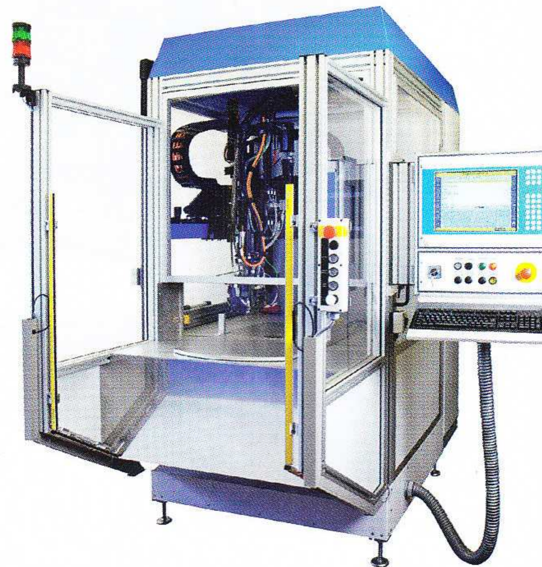
Fig. 4. Smart - DM 402 dosing cell for gasketing, adhesion bonding and casting (figure: Sonderhoff)
