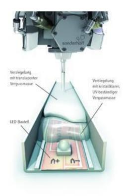
2 layers' casting application with transparent and opaque potting systems Fermadur®
