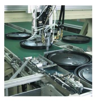
Foam gasket application on plastic barrel lids with Fermapor K31 polyurethane sealing using a Sonderhoff mixing and dosing system
