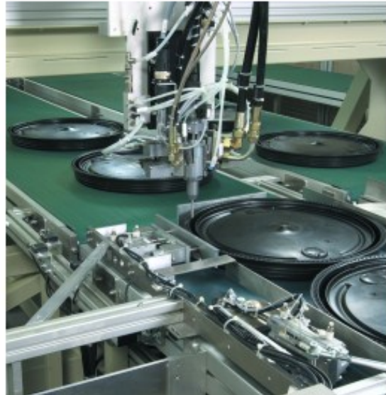
Foam gasket application on plastic barrel lids with Fermapor K31 PU sealing using a Sonderhoff mixing and dosing system
