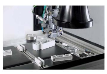
The optics in the new dispensing cell automatically recognises different component sizes and shapes despite arbitrary position on the transfer conveyor.
