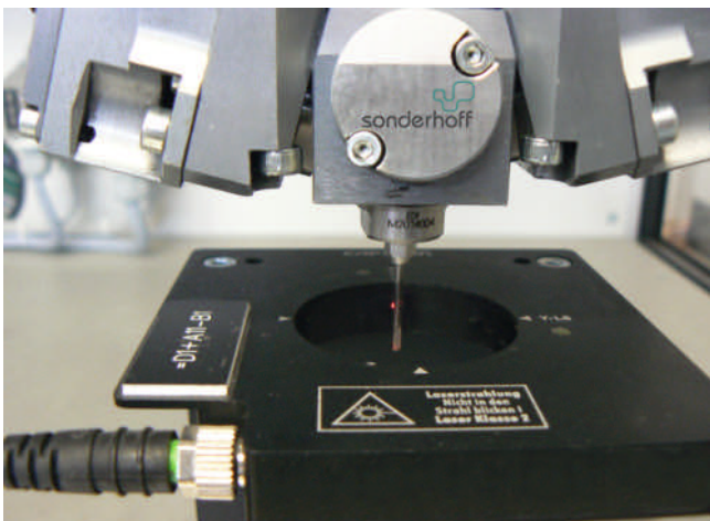
Fig. 3. Two laser sensors at a right angle to one another check whether the application nozzle is correctly positioned
