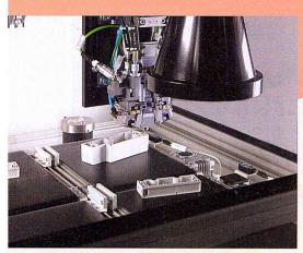
Due to the optionally equipped automatic part recognition in the dispensing cell the fully automatic sealing process with Sonderhoff foam gasket and potting products is also possible in the case of a random parts feed. (photo: Sonderhoff)
