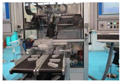
The high-performance optics in the new dispensing cell SMART - DM 402 automatically recognizes different component sizes and shapes despite arbitrary position on the transfer conveyor.
