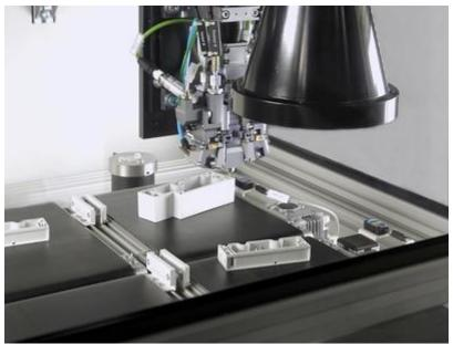
The intelligent part recognition system verifies the arbitrary position of the components on the transfer conveyor and automatically recognizes the different component sizes and shapes.
