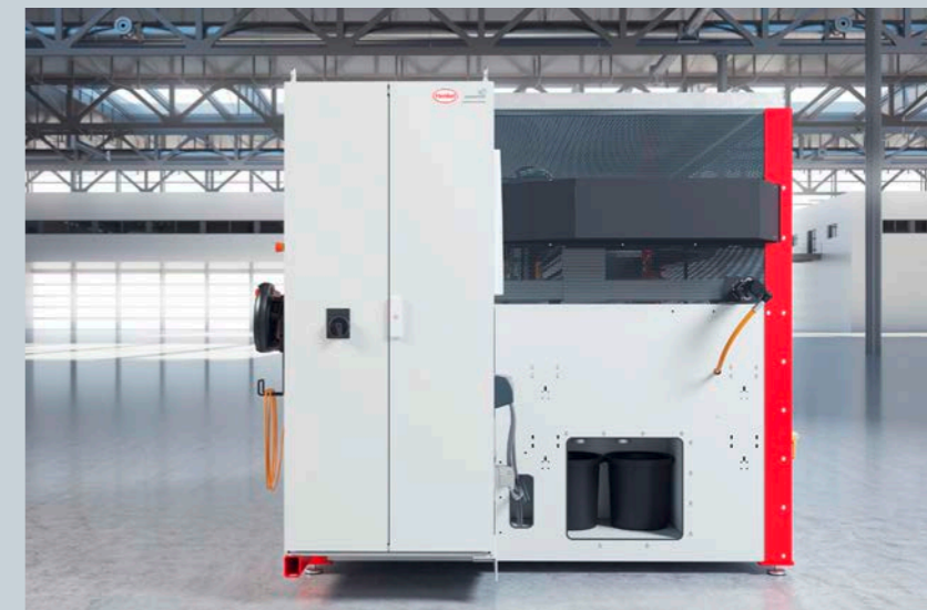
The front side (right) of the SONDERHOFF 3E FLEX dosing cell shows the switch cabinet attached to the cell chassis for controlling the dosing machine, to the left of which you see the holder for the MP 2 mobile panel, and to the right the opening for removing the filling shot and rinse water containers
