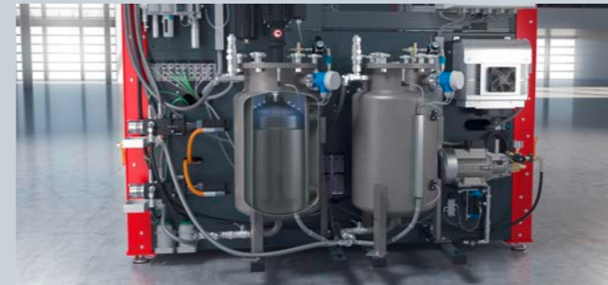
Compressed air cushion acts on material surface
