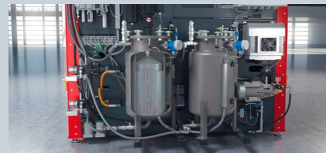
Material is continuously conveyed from the bottom of the pressure tank through a riser pipe and fed back onto the conical surface as a thin film. Due to the air loading, the density changes and the material becomes lighter in color.
