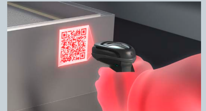
Hand-held scanner for selecting the CNC and dispensing program
