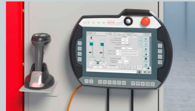
Multi-functional MP 2 mobile panel with integrated touchscreen
