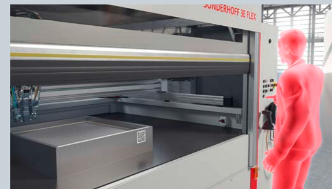
To remove one or more parts after dispensing, the high-speed door opens automatically or the operator opens it by pressing a button.
