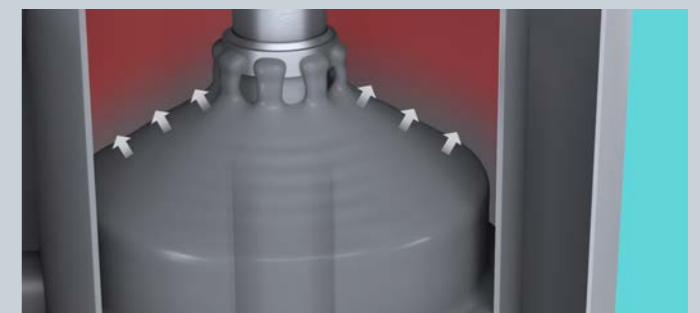
Material is continuously conveyed from the bottom of the pressure tank through a riser pipe and fed back onto the conical surface as a thin film. This process continuously reduces and completely dissolves air bubbles in the material.
