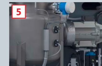
Capacitive sensors for filling level regulation
