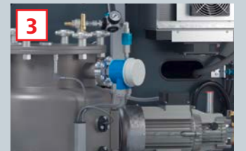
Overfilling protection for the use of an optional refilling station
