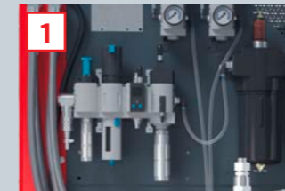
Compressed air connection, dryer and maintenance unit
