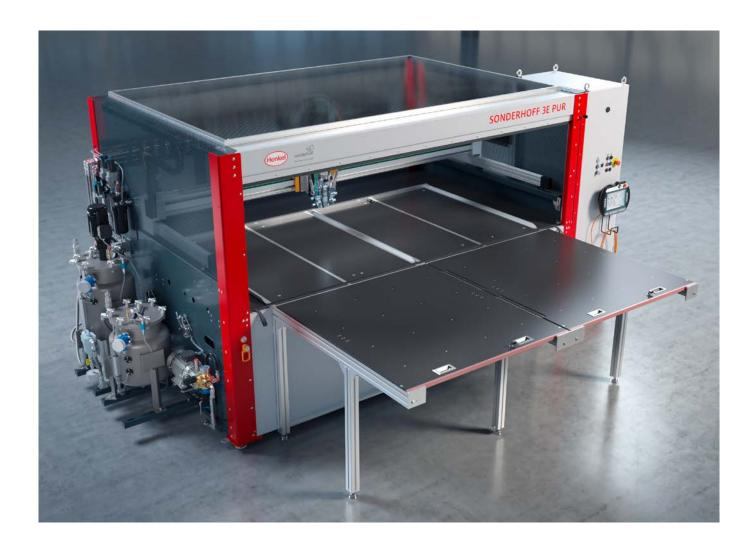
The SONDERHOFF 3E PUR dosing cell offers an attachable sliding table with manually shifting mounting plates as an alternative option for placement and processing of industrial parts for sealing, bonding, or potting. With this solution, a machine operator loads the two mounting plates with the parts in an alternating sequence. The parts are positioned in workpiece fixtures, which are fastened on the mounting plates made of coated multiplex.
