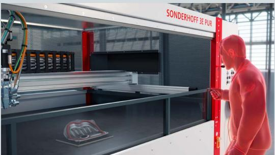
To remove one or more parts after the dispensing process, the machine operator opens the lifting door using either the hand strap mounted there or the lever.
