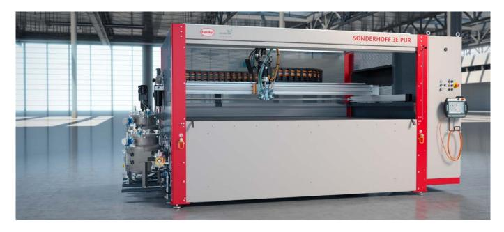
The SONDERHOFF 3E PUR dosing cell comprises the MK 825 BASIC precision mixing head for 2-component products with high-pressure water rinsing for mixing chamber cleaning. In the mixing head the material components are mixed dynamically, and the material system to be applied to the part is dosed in precise quantities. The MK 825 BASIC enables dosing from 0,2 to 3,0 g/s with continuously adjustable, asymmetrical mixing ratios from 10:1 to 1:2 and a dosing accuracy of ±1%.
