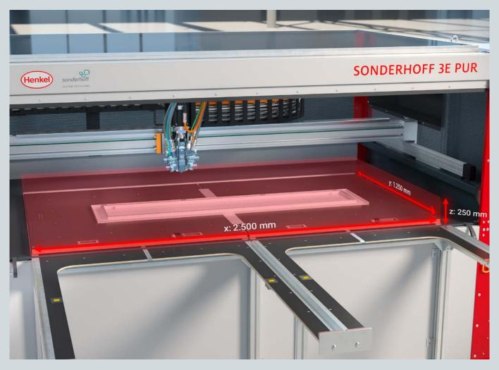
In order to be able to produce oversized components with a maximum dimension of 2,500 x 1,250 x 250 mm (x/y/z), the two sliding table plates are joined together to form one large mounting plate.
