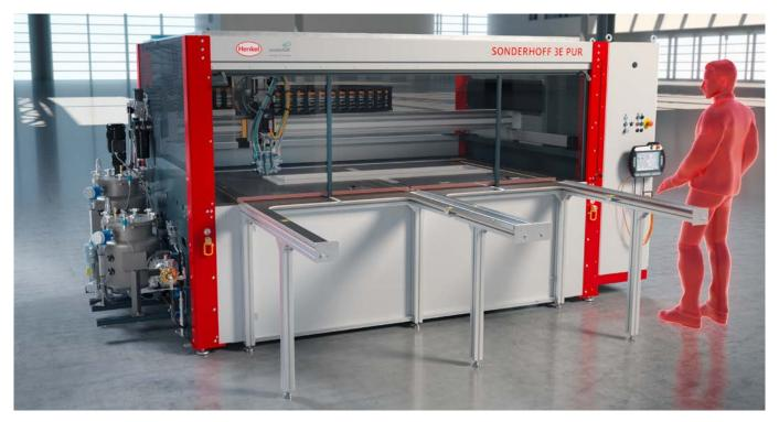
For material application on oversized components, the two mounting plates can be connected to form a single large sliding table.
