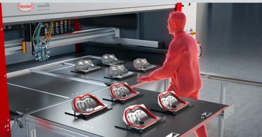
After the dispensing application, the machine operator opens the lifting door and pulls the sliding table with the finished parts out of the working area for removal.
