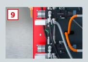
Precision gear pumps with flow rate 0.75 ccm/rev (material component A) and 0.3 ccm/rev (material component B)
