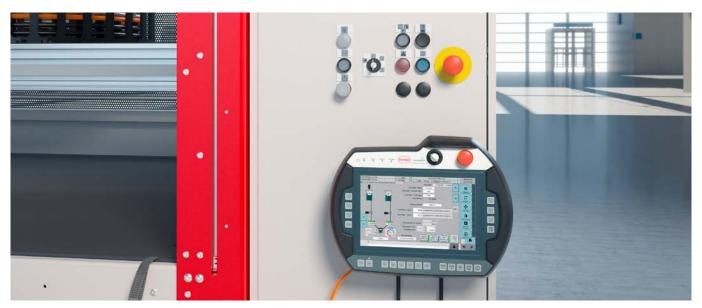
MP 2 mobile panel and above it the operating mode control panel, e.g. key switch for operating mode preselection with selection for the operating modes of Setup / Stand-by / Manual / Automatic, warning lights and EMERGENCY STOP, part of the tried-and-tested SONDERHOFF SAFETY concept.
