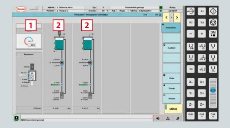
Shows the two material components, the tank level, the pump speed, the line pressure downstream of the pump, the mixing head temperature, the dispensing time (seconds), the discharge line (g/s) and the reactivity of the material (pot life in seconds)
