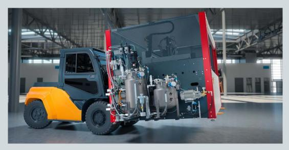
The dosing cell is removed from the transport container, set up and connected: place, plug & work. All features are arranged on a single chassis so that the dosing cell can be changed over very easily in production.
