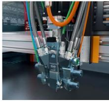
Standard equipment: MK 825 BASIC precision mixing head for 2 components, with high-pressure water rinsing
