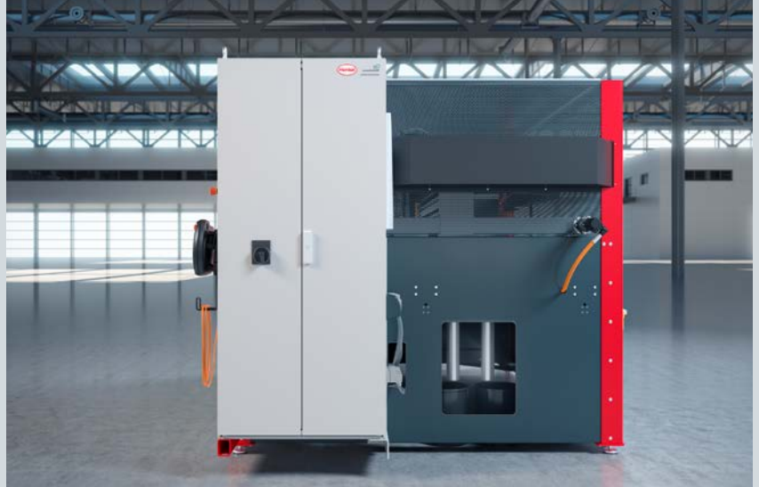
Right side of the SONDERHOFF 3E PUR dosing cell shows the switch cabinet attached to the cell chassis for controlling the dosing machine, to the left of which you see the holder for the MP 2 mobile panel, and to the right the opening for removing the filling shot and rinse water containers
