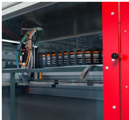
Half-open lifting door shows MK 825 BASIC precision mixing head and energy chain
