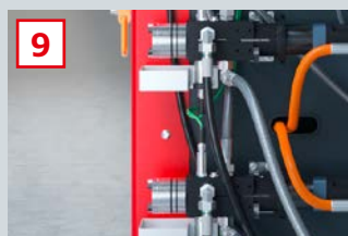
Precision gear pumps with flow rate 0.75 ccm/rev (material component A) and 0.3 ccm/rev (material component B)
