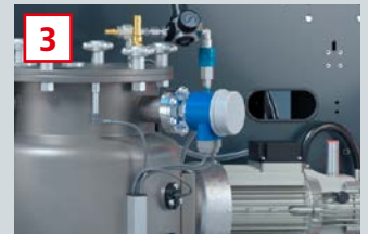
Overfilling protection for the use of an optional refilling station
