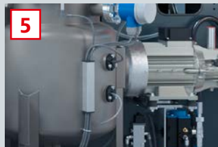
Capacitive sensors for filling level regulation
