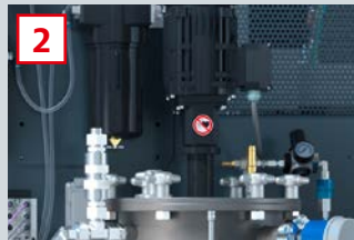
Agitator for homogenization of the material component A
