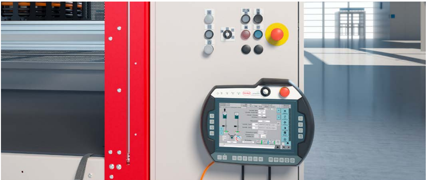
MP 2 mobile panel and above it the operating mode control panel, e.g. key switch for operating mode preselection with selection for the operating modes of Setup / Stand-by / Manual / Automatic, warning lights and EMERGENCY STOP, part of the tried-and-tested SONDERHOFF SAFETY concept.
